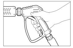
**Step 3** With the engine running, pull trigger to operate unit: Liquid detergent is drawn into the unit and mixed with water. Apply detergent to work area. Do not allow detergent to dry on surface.
